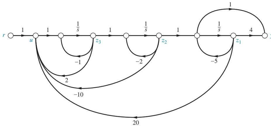
**FIGURE 12.10** Designed system with state-variable feedback for Example 12.4
