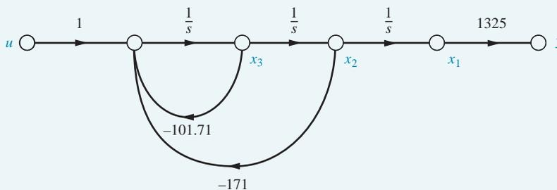
**FIGURE 12.24** Signal-flow graph for  $G(s) = 1325/[s(s^2 + 101.71s + 171)]$
