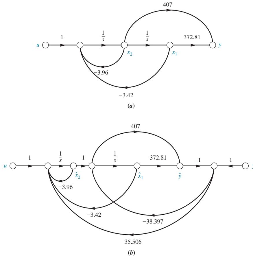
**FIGURE 12.20** a. Plant; b. designed observer for Example 12.9
