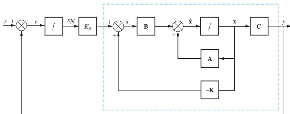
**FIGURE 12.21** Integral control for steady-state error design
