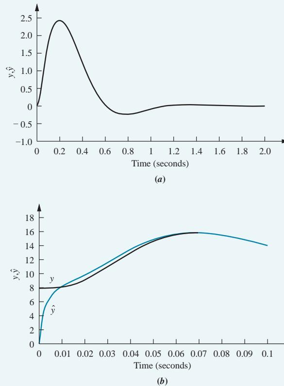
**FIGURE 12.27** Designed response of antenna azimuth position control system: **a.** impulse response—plant and observer with the same initial conditions,  $x_1(0) = \hat{x}_1(0) = 0$ ; **b.** portion of impulse response—plant and observer with different initial conditions,  $\hat{x}_1(0) = 0.006$  for the plant,  $\hat{x}_1(0) = 0$  for the observer
