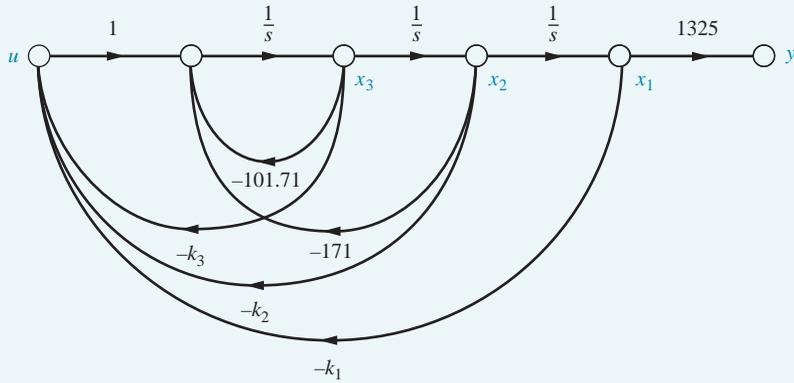
**FIGURE 12.25** Plant with state-variable feedback for controller design
